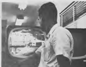
LAGO IS on television. It's the company's own television station and is confined to San Nicolas Harbor and approaching sea lanes. The closed circuit system has been installed in the Marine Department's sight approaching tankers. E. A. Halley of the Instrument Shop adjusts focus. LAGO NA television. Pero ta television di compania mes esaki ta, y e ta traha solamente den haaf di San Nicolas y refugio di laman. E sistema di television astra e wordo instalá den departamento di marina pa mira e tankeran cu ta zecando aki banda.
